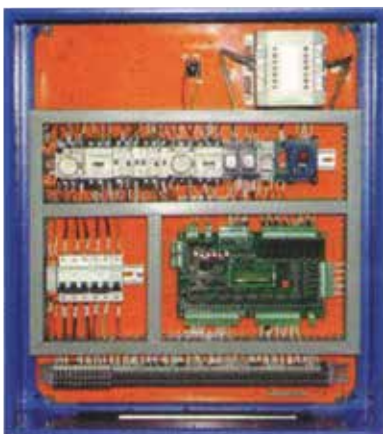
Traction ARD (Automatic Rescue Device)
